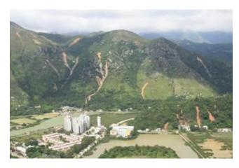
This was one of the most notable storms to have occurred in Hong Kong in several decades, with a 4-hour rolling rainfall equated to a return period of 500-1000 years. A number of the landslides developed into major debris flows, with significant secondary entrainment and long run out distances. Such hazards were underrepresented in the existing data sets at that time.
